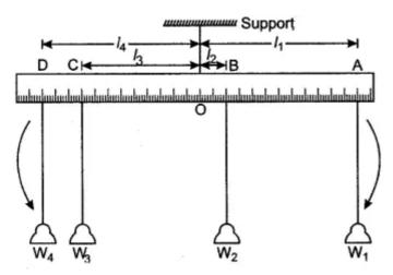
Let  $W_1$ ,  $W_2$  and  $W_3$ ,  $W_4$  be the weights suspended and  $I_1$ ,  $I_2$  and  $I_3$ ,  $I_4$  are respective lengths. The weights  $W_1$  and  $W_2$  tend to turn the scale clockwise while the weights  $W_3$  and  $W_4$  tend to turn the scale anti-clockwise.
