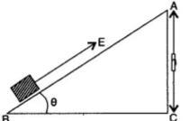
An inclined plane is usually a smooth, flat rigid surface inclined at an angle ( $\theta$ ) to the horizontal. It is used to raise heavy loads with relatively small force. The longer the slope, the smaller is the effort needed.
