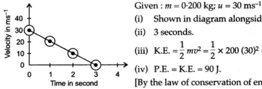
Shown in diagram alongside. (iii) K.E.  $=\frac{1}{2}mv^2 = \frac{1}{2} \times 200 \ (30)^2 = 90 \text{ J.}$ (iv) P.E. = K.E. = 90 J.
